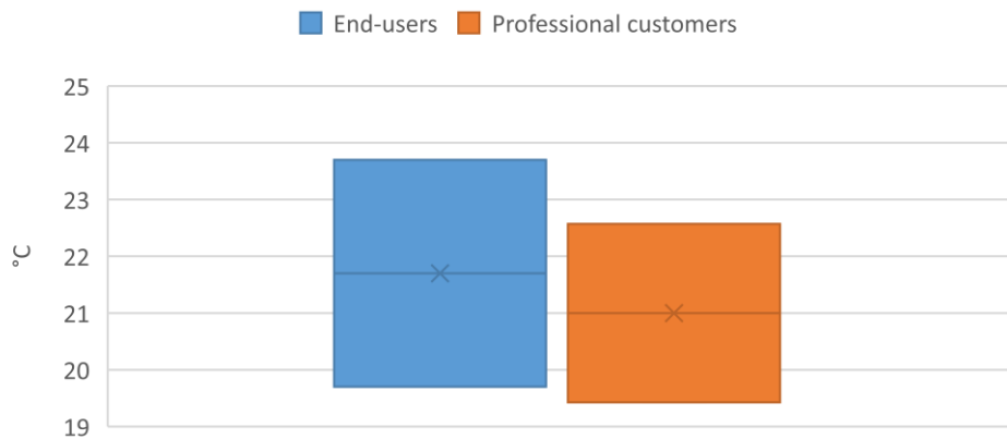
Figure 38: Mean preferred indoor temperature and accepted deviation from preferred temperature (Italian demo site)
