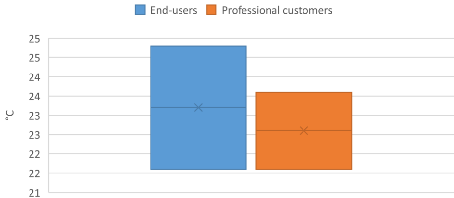
Figure 23: Mean preferred indoor temperature and accepted deviation from preferred temperature (Croatian demo site)
